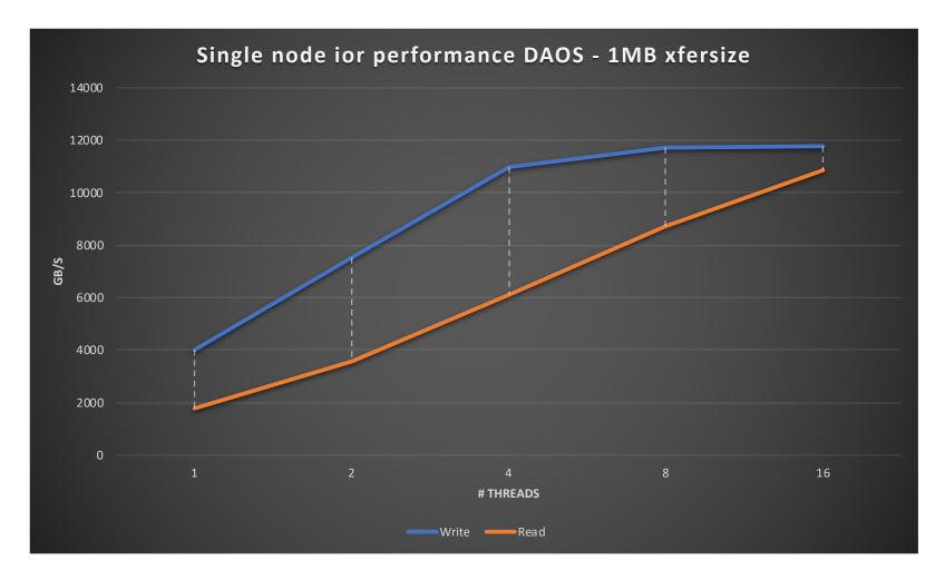
• Scale linearly with the number of tasks until client OPA link is saturated.
