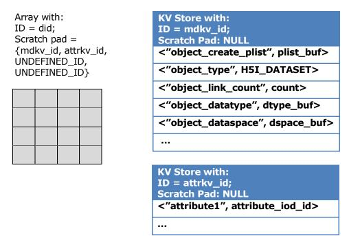
The datatype and dataspace objects can be retrieved from the binary buffers stored in the metadata KV store by calling *H5Tdecode()* and *H5Sdecode()* respectively.
