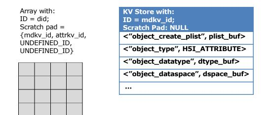
Attributes always are created attached to an object (File, Group, Dataset, or Named Datatype). Objects can have multiple attributes attached to them. As we have shown previously, each type of those objects has a separate KV store for storing attributes in their scratch pad. The Key will hold the attribute name which has to be unique for a particular object (i.e. an object cannot have two attributes with the same name), and the value will hold the IOD ID for the actual attribute object.
